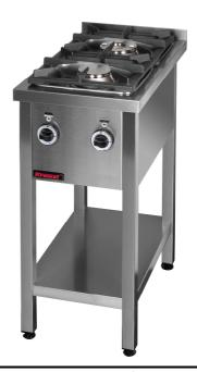
**Description:** Gas cookers are made of high-grade stainless steels. Working plate made of AISI 304 stainless steel. Burners and grates made of cast-iron. Removable bowls for liquids ejected when cooking under burners. Adjustable burner power. Cooker is equipped with pilot burner with flame safety device. Cooker is equipped with storage shelf. Grill adapters (smooth, grooved), reduction adapters and Wok grate can be used.
